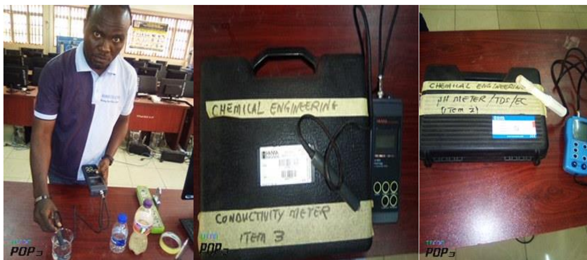
Figure 3. Mobile Water Quality Testing Using Hannah Instruments (i.e. pH Meter - code: HI9812-5) and (Multi-range Conductivity Meter - code: HI9033).
