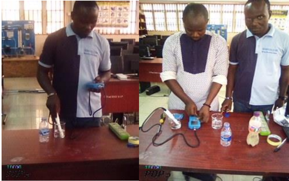
Figure 3(continue). Mobile Water Quality Testing Using Hannah Instruments (i.e. pH Meter - code: HI9812-5) and (Multi-range Conductivity Meter - code: HI9033).
