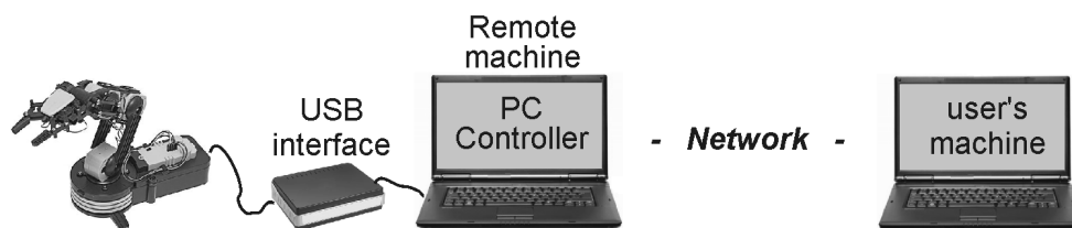
Figure 3. The scheme of remote controlling for simple small models of robots
