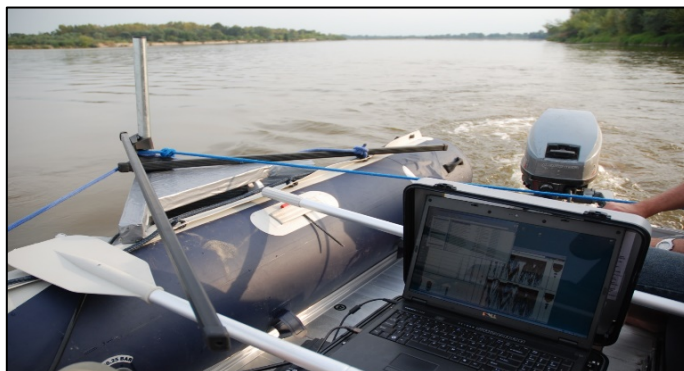
Fig. 8. WULS integrated hydrographic system in operation [4]
