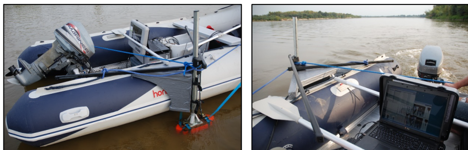
Fig. 2. Hydrographic set comprised of a sonic sounder integrated with a DGPS receiver
