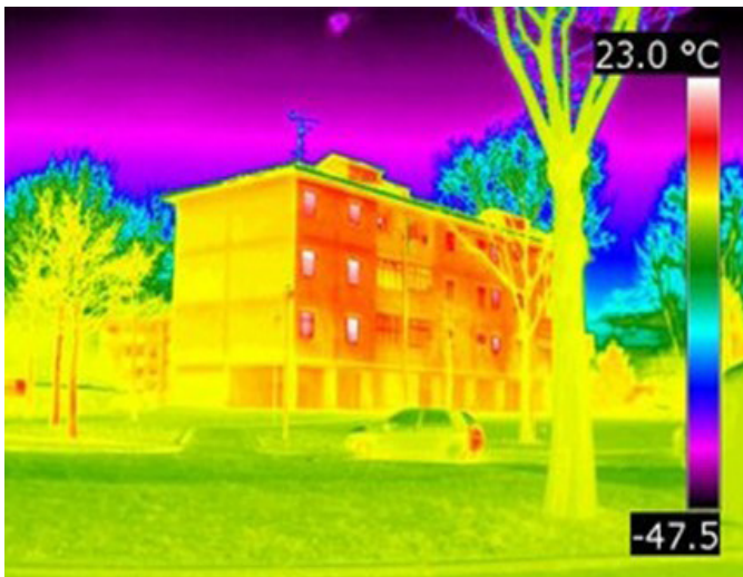
Fig. 3. Photography of the 'building plate', made with the use of thermal imaging camera [12]
