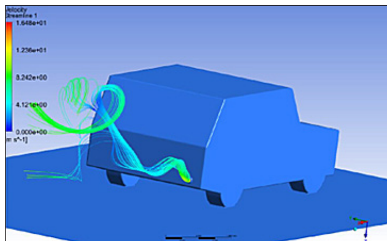
Figure 2. Exhaust gas tumble at a cross wind
