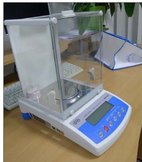
Figure 7. Laboratory equipment for determining the mass of loose material particles
