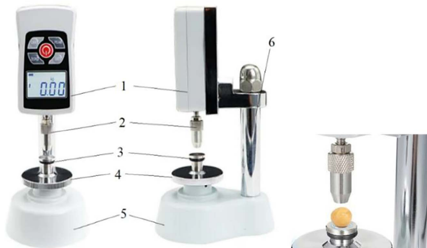
Figure 8. Digital pressure gauge (Tester AGW-3): 1– digital unit; 2 – pressure head; 3 – loading platform; 4 – flywheel of the platform; 5 – base; 6 – column
