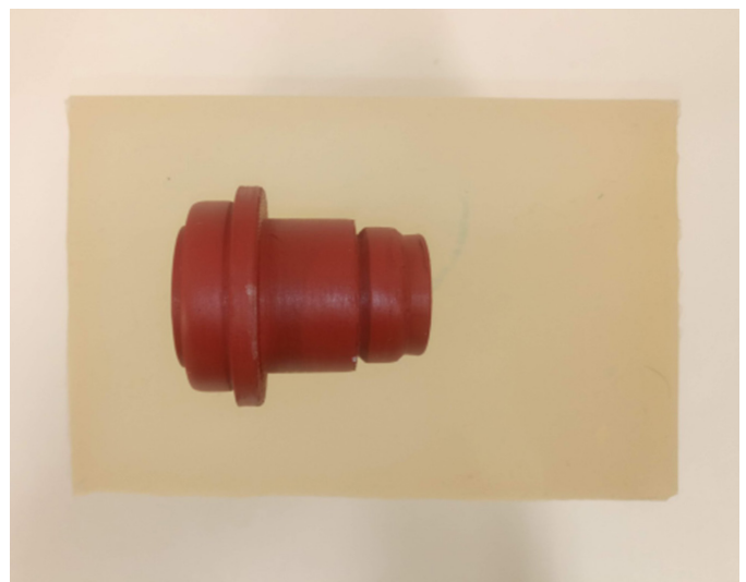
Fig.10. Wax castings of valve body parts
