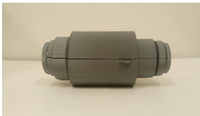
Fig. 9. Valve prototypes after the destructive bench testing process – from the left, the ABS valve and the PLA valve
