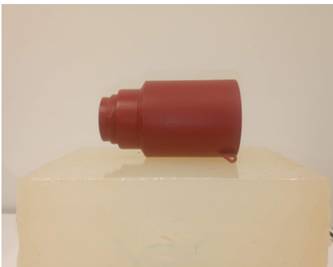
Fig.10. Wax castings of valve body parts
