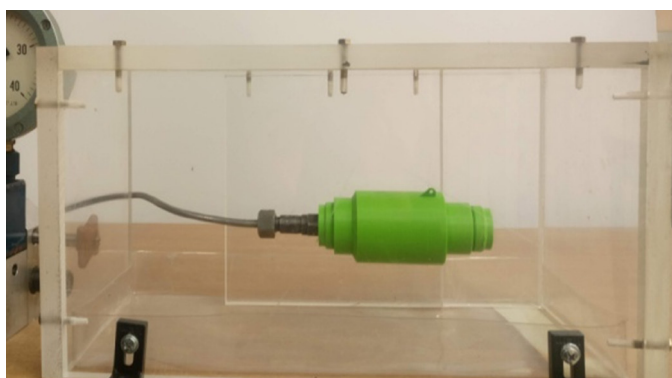
Fig. 8. Destructive bench testing process – from the left, the ABS valve and the PLA valve
