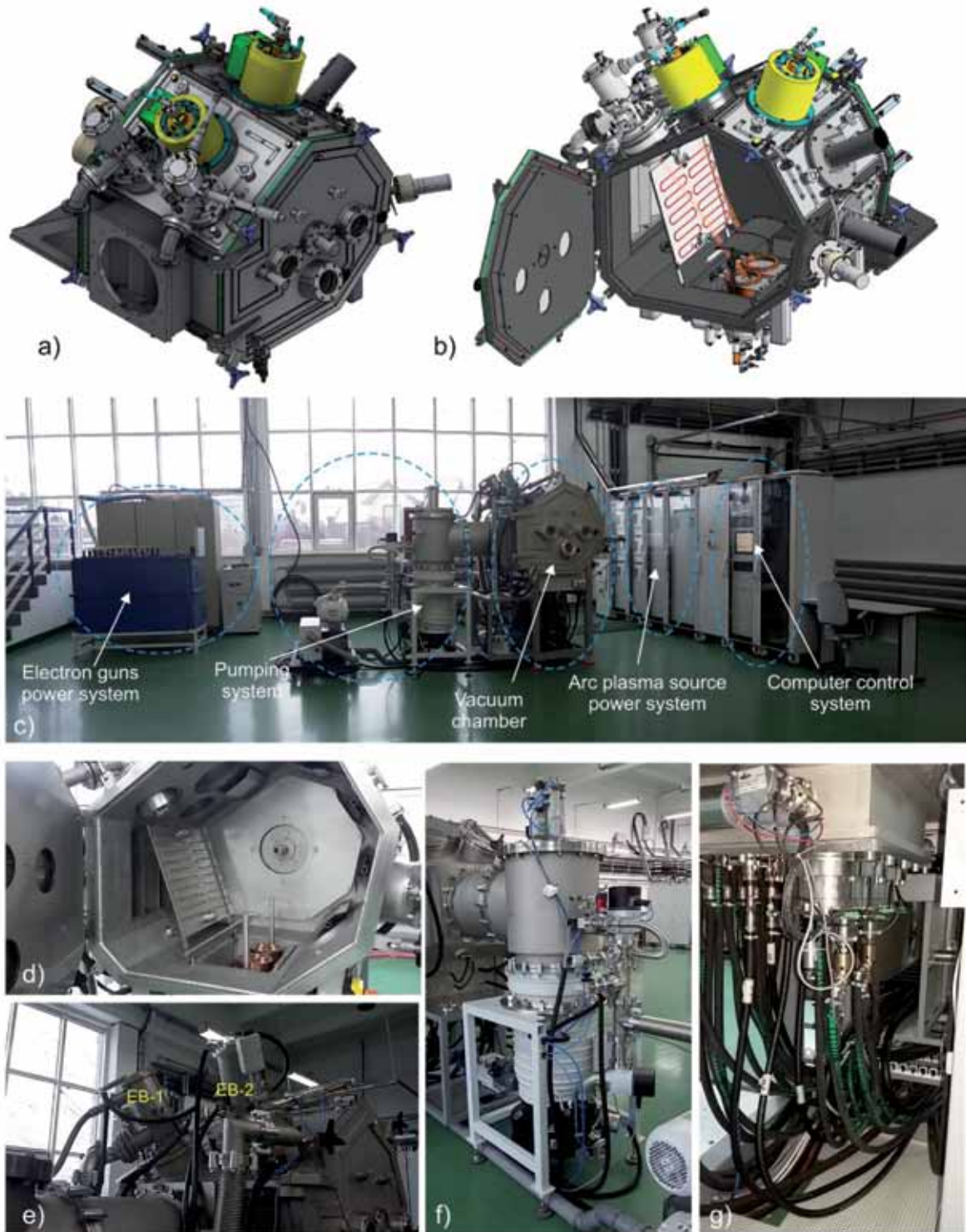
Fig. 5. The EB-Dual BEAM technological device designed and built at ITeE – PIB in Radom (Poland), adapted to the process of evaporation materials by electron beam, using two electron guns: (a, b) technical design, (c) view of the device with the description of individual functional systems, (d) the inside of the process chamber, (e) view of two electron guns mounted on the process chamber, (f) pumping system, (g) water cooling system of the process chamber
