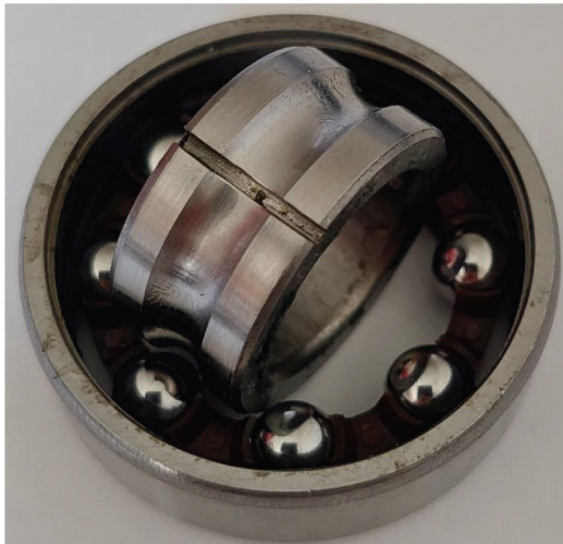
Figure 21. Bearing (6203-Z) with a rectangular spall (width s = 1.1 mm) perpendicular to the inner raceway. By utilising a polyamide cage, the bearing could be dismantled without damage.
