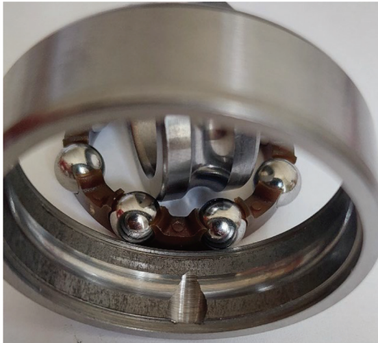
Figure 22. Bearing (6203-Z) with a fault resembling a parabolic spall (width s = 3.3 mm) on the outer ring.
