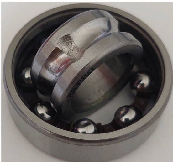
Figure 23. Bearing (6203-Z) with a fault resembling a parabolic spall (width s = 3.4 mm) on the inner ring.
