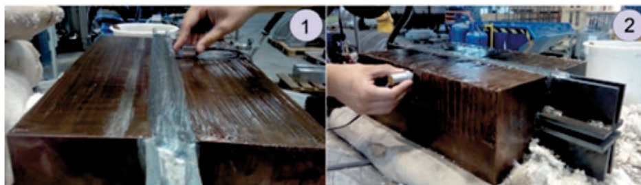
Fig. 5. Examination of the sample with the ultrasonic method: 1) 45 ° angle head, 2) A straight head
