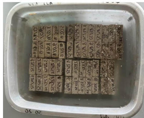
Fig. 5. Thickness swelling and water absorption test samples.
