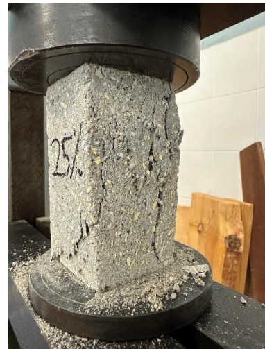
Fig. 4. Compressive strength test sample during testing.
