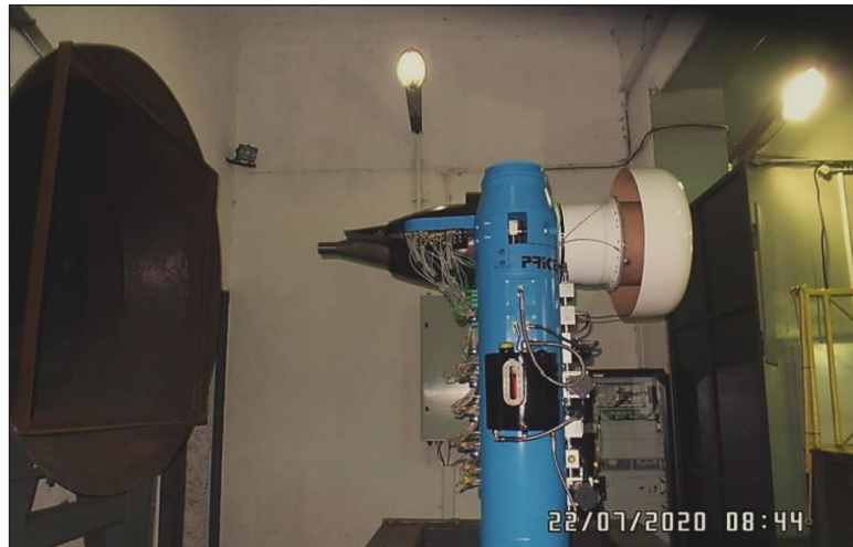
Fig. 6. DGEN 380 engine integrated on a static thrust stand
