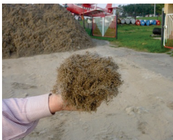
Fig. 3. Mixture of sand, native soil and polymer fibres [12]
