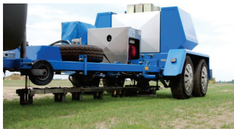
Fig. 11. HWD deflectometer test
