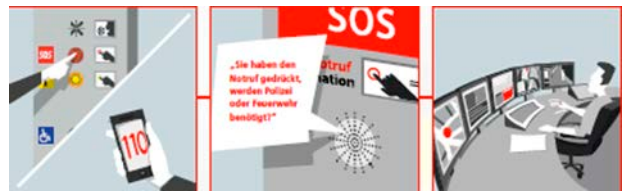
Figure 2. Operational diagram of the SOS (NOTRUF) bollard panel at a Berlin metro station (BVG, 2023)
