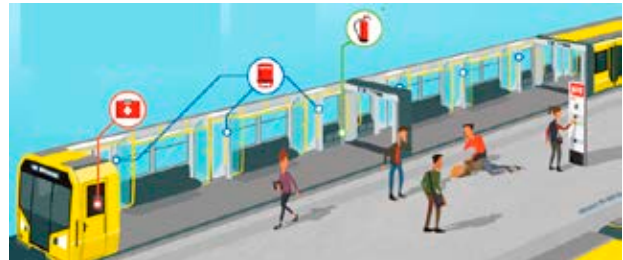
Figure 1. Location of emergency buttons, fire extinguisher, and first aid kit in metro trains and the SOS (NOTRUF) bollard panel at the station (BVG, 2023)
