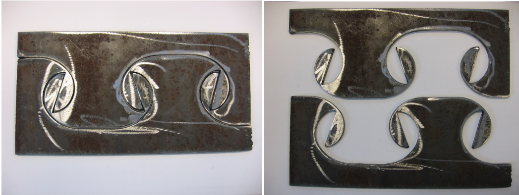
Figure 15: Production technology of the clothoidal symmetrical shape without problems with overheating of the steel (the process results in a shape with a more extensive upper part of the steel dowel compared to the initial CL shape): the idea of cutting line (at the top) and the first-cut sheet fragments delivered by the contractor for acceptance of the technology (pictures taken in Wrocław on 10.17.2008)
