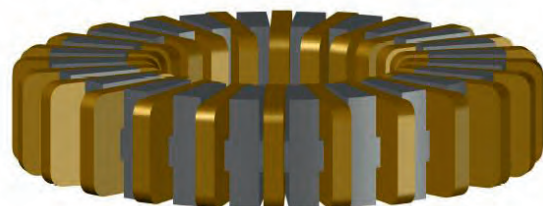
Fig. 12. 3D model of disc stator with axial winding
