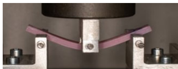
Fig. 3 A specimen made of NextDent Denture 3D+ polymer, situated between the branches of the testing machine
