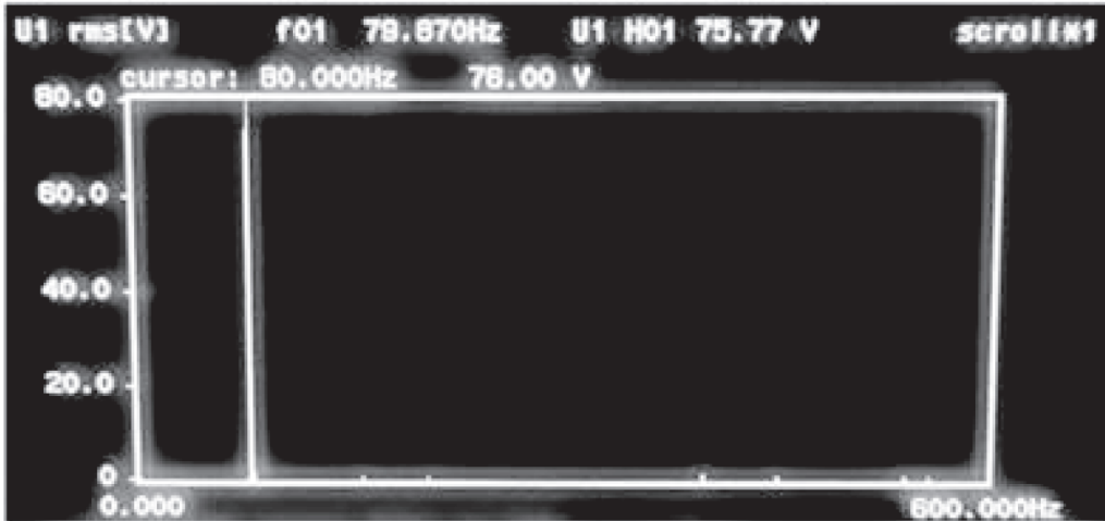
Figure 12. Experimental result: Low-frequency harmonic spectrum of the output line-to-line voltage analysed through the Norma D6200 Power Analyser manufactured by LEM NORMA GmbH. Shoot-through duty ratio: 0.16. Desired output frequency: 80 Hz. Modulation index, m = 0.8 . Three-phase AC voltage at the input of the diode bridge rectifier: 100 V (line-to-line), 50 Hz.
