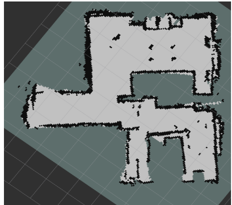
Fig. 4.2. Map generated using the RTAB-map algorithm
