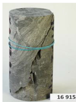
Fig. 7. Fracture pattern comparison for compression of Mohr-Coulomb sample with different shear strength set.
