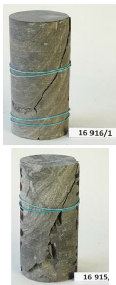
Fig. 13. Fracture pattern comparison for compression of ubiquitous joint Mohr-Coulomb sample with different shear strength sets of a weak plane.
