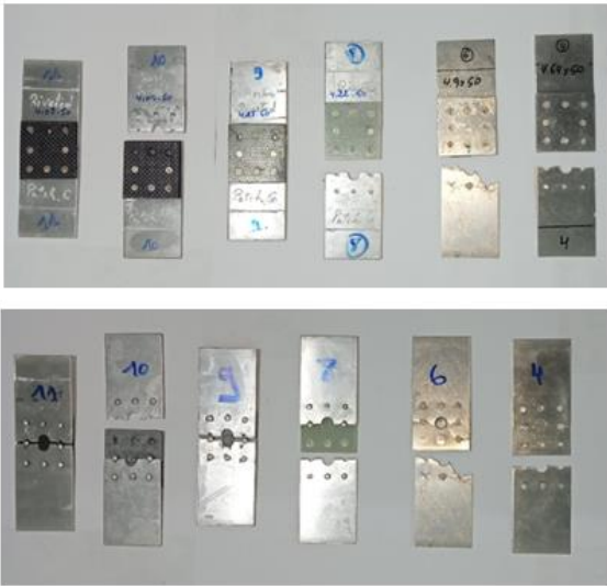
Fig. 20. Damage to notched plates repaired by different types of patch using hybrid repair processes (bonding/riveting)
