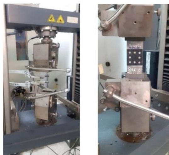
Fig. 9. Illustration of the test bench for tensile tests
