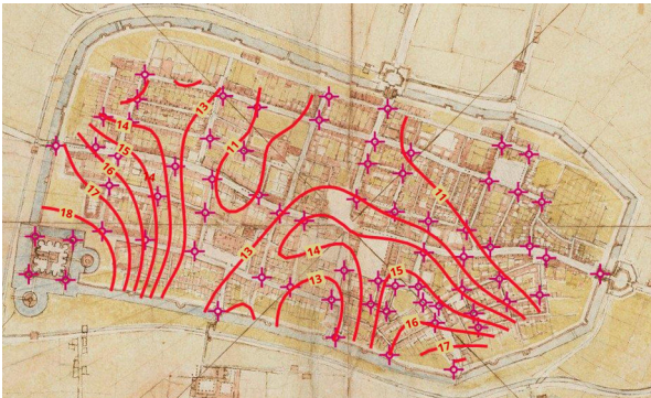
Figure 16. Isolines of local map rotation angles (at the interval of 1 degree) on Leonardo da Vinci's map (Royal Collection Trust / © His Majesty King Charles III 2023) and on the modern OSM map
