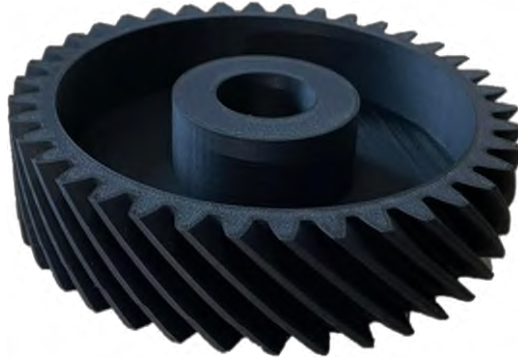
Fig. 2. Prototype of an oil centrifuge wormwheel made by FDM method
