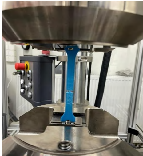
Fig. 7. An example of a sample after a static tensile test
