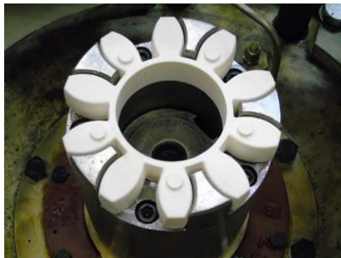
Fig. 1. An insert of the claw thruster clutch made by the FDM method
