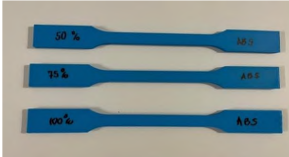
Fig. 6. Examples of samples prepared for the static tensile test
