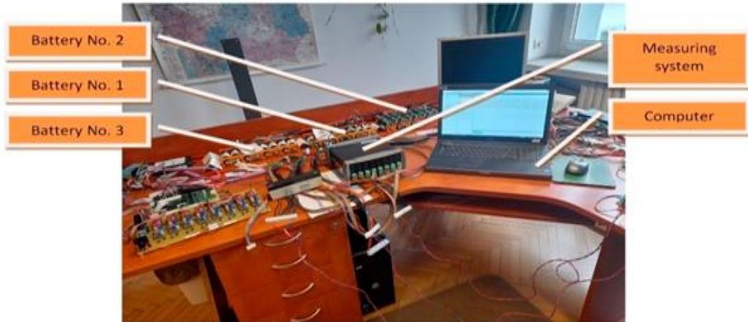
Fig. 6. Station for measuring and recording data (Battery 1 - with a battery for the active BMS battery, Battery 2 - with a battery for the active BMS battery, Battery 3 - with a passive BMS)
