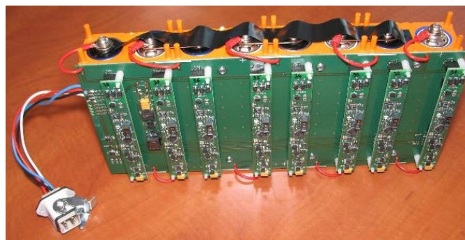
Fig. 3. BMS system installed on the cell pack
