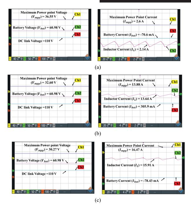
Figure 9. System performance during (a) low, (b) mid and (c) high irradiance level.
