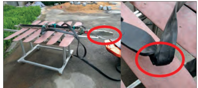
Fig. 1. Damage to the rudder and umbilical cable of a wave glider caused by fishing nets
