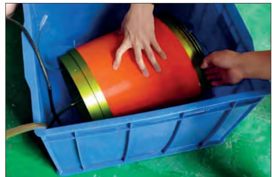
Fig. 10. Test of buoyancy regulation system module
