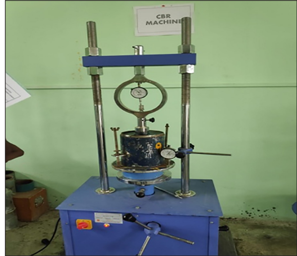
Figure 3. CBR test on samples
