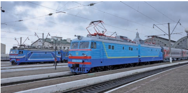
Fig. 8. Lviv Main Station is a voltage switching station – individual sections have the option of being powered by either alternating or direct current: VL40-1457-1 (1520 mm, 25 kV 50 Hz) with a long-distance train to Kyiv (UZ carriages) and VL10-1478 (1520 mm, 3 kV DC) with a long-distance train as the one Chop – Kyiv – Moscow (RZD carriages) (28.04.2013) [photo: M. Graff].
