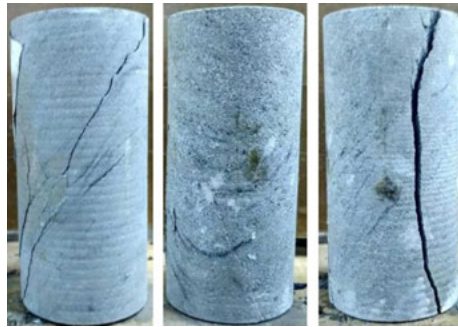
Fig. 12. Rock samples obtained on-site and post-fracture characteristics
