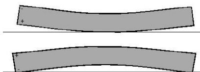
Fig. 5. Scheme of deformation of a concrete slab depending on the temperature distribution inside it
