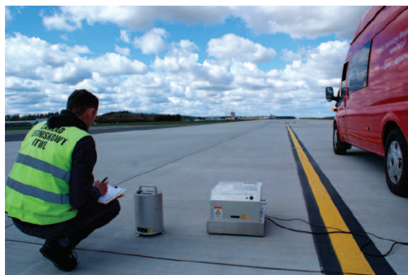
Photo 1. Measurements made with ElaTexture and CTM stationary devices
