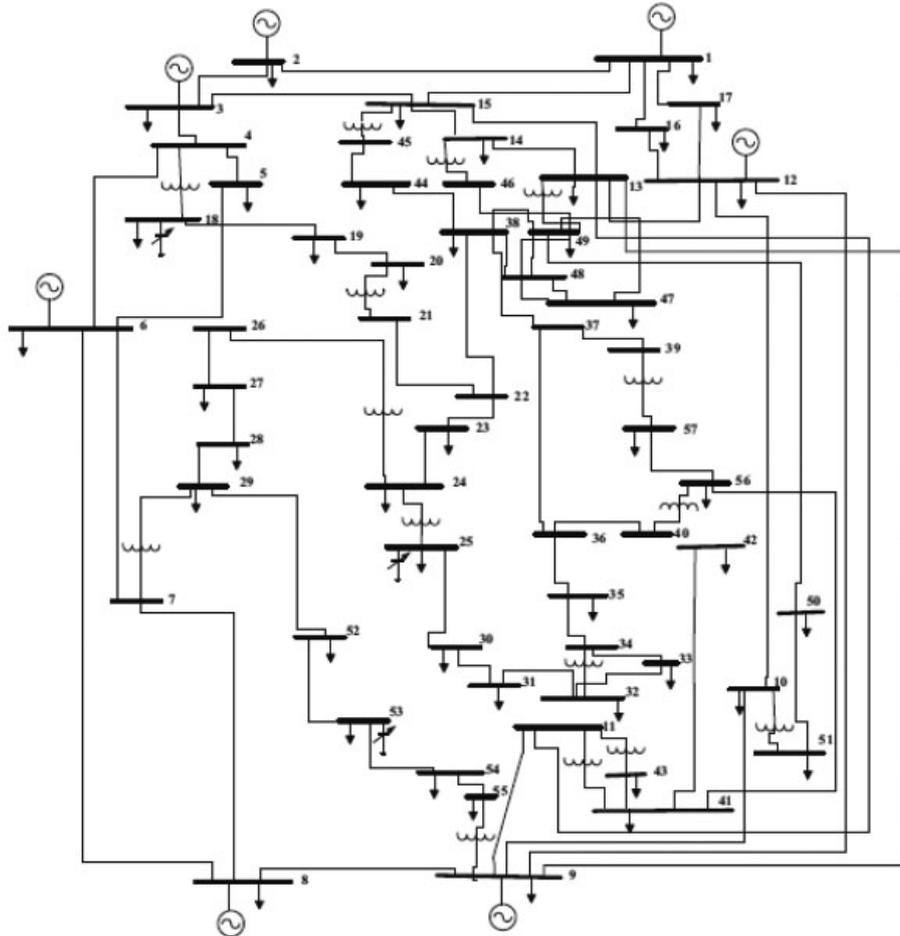
Fig. 5. Single-line diagram of IEEE57-bus power system [27]
