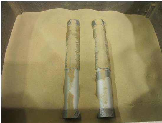
Fig. 4. The sand layer reaches the center line of the tunnel to be excavated
