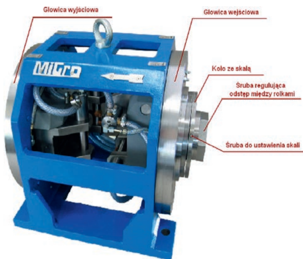
Fig. 1. Cassette for mounting sets of rollers [9]
