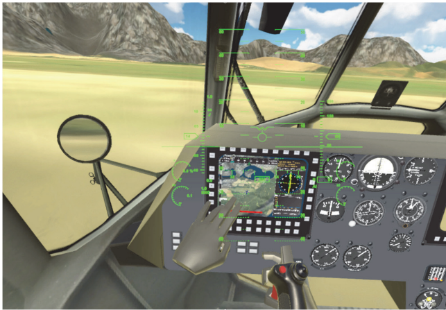
Fig. 6. Mismatch between the position of digital twin of the control stick and the virtual hand of the operator
