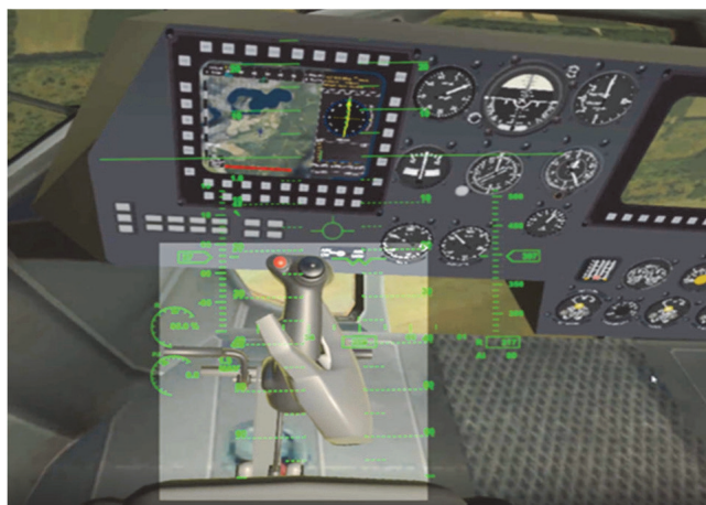
Fig. 8. Reconciling the position of the virtual hand and the digital twin as a result of MR calibration (hand and joystick on the light background)
