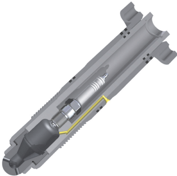
Fig. 7. Prechamber in Waukesha AT series engine (yellow – chamber gas supply)
