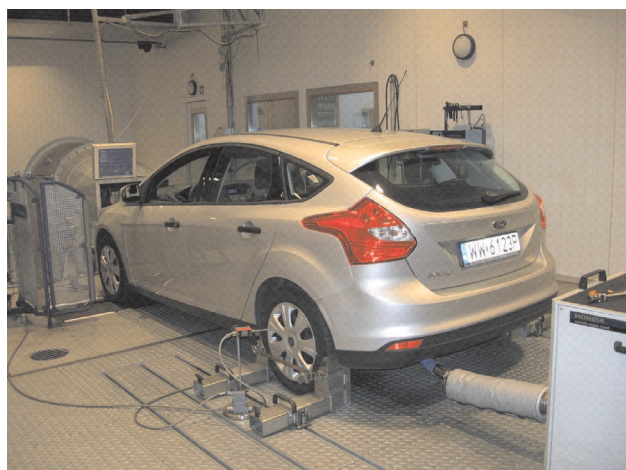
Fig. 4. BOSMAL Emission Testing Laboratory (cell 2) – internal view of the climatic chamber
