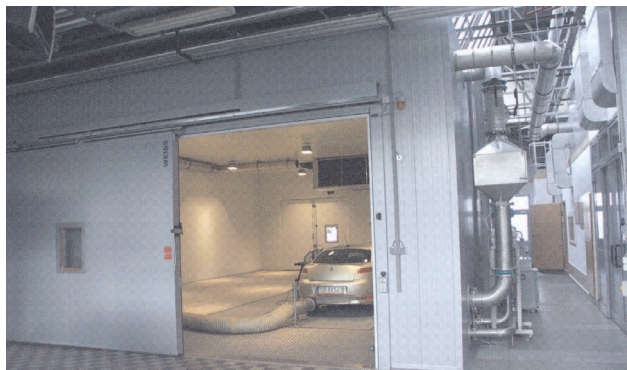
Fig. 5. BOSMAL Emission Testing Laboratory (cell 2) – external view of the climatic chamber
