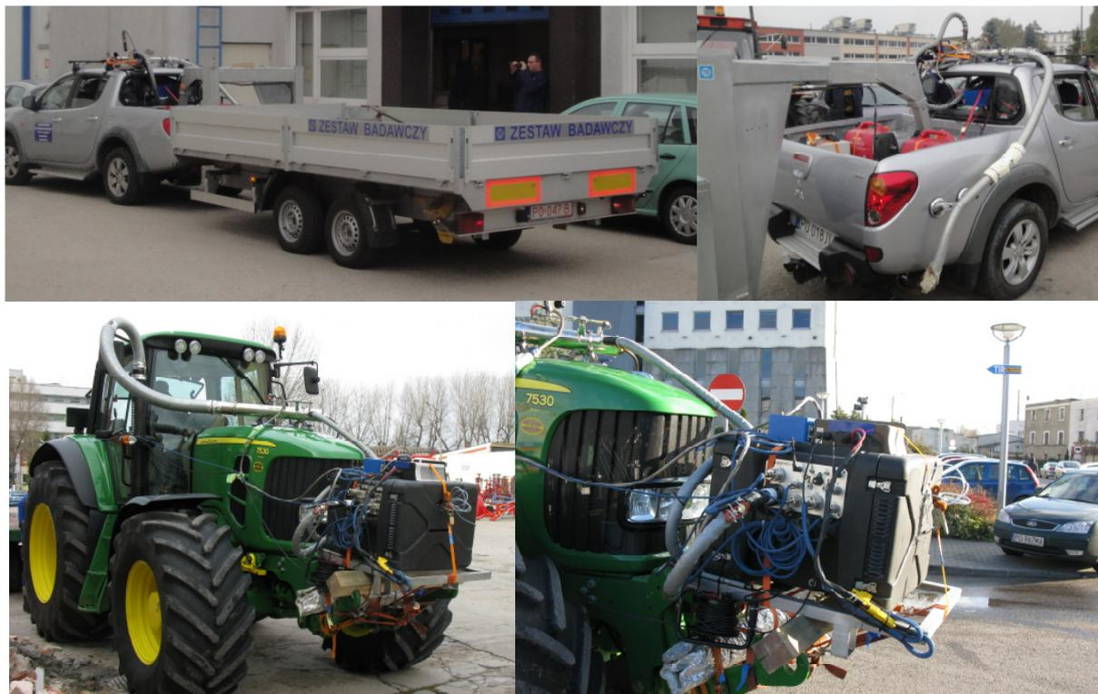
Fig. 1. View of the vehicles and the measuring devices
