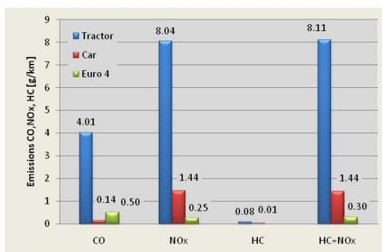
Fig. 4. Comparison of the road emission of the utility vehicle and the farm tractor during the tests under real operating conditions
