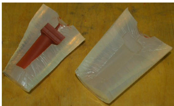
Fig. 4. Silicone mold and manufactured wax model
