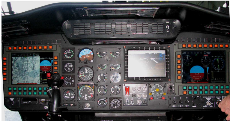
Fig. 3 The cockpit with components of the ITWL-developed integrated communication system built into the W-3PL "Głuszc" helicopter
