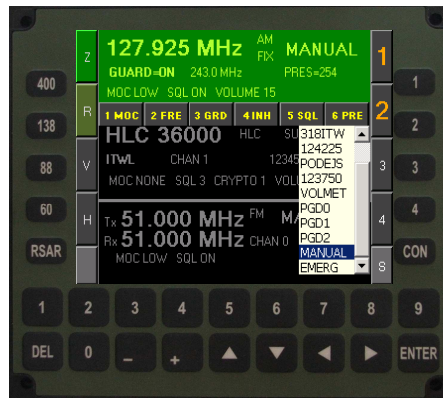
Fig. 2 The PSL-1 control panel included in the ITWL-developed integrated communication systems
