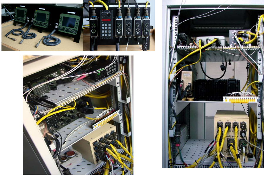
Fig. 5 The testing station with communication system's components (left) and control items (right), constructed and developed at the ITWL's Division for Avionics
