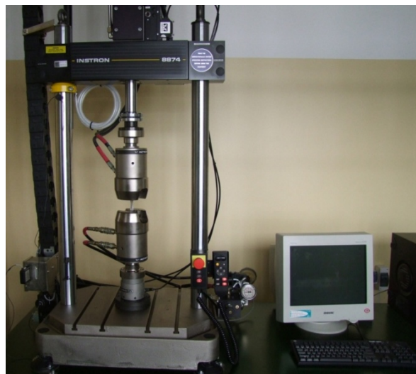
Fig. 5. Servo-hydraulic material-testing machines, Instron 8874
