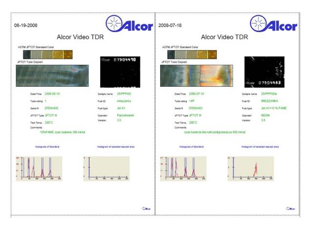
Rys. 2. Example spectrum of tube deposit rating after thermal stability testing cycle course (cycle I and VI)
