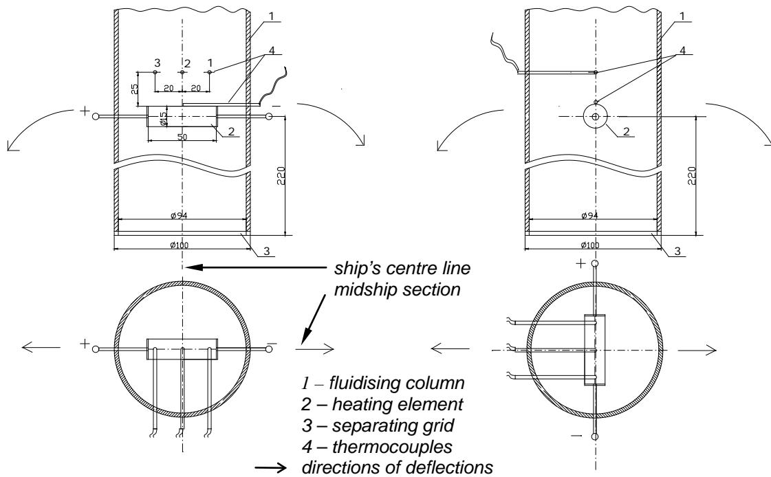
*Fig. 1. Diagrams of the positioning of heating element and distribution of thermocouples*
