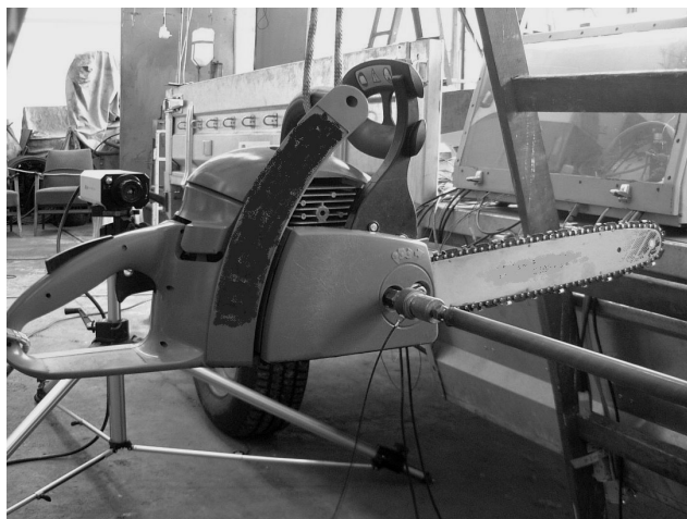
Fig. 9. The chain saw at the station for experimental modal identification
