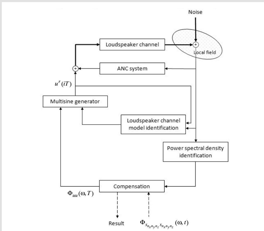
**Fig. 3.** Block diagram of an acoustic local field adaptive synthesis and generation system
