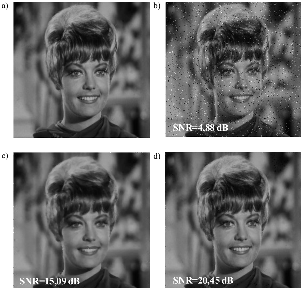
Fig. 3. Restoration of noise-corrupted Zelda image: a) original image; b) noisy image; c) median filtration; d) the new approach
