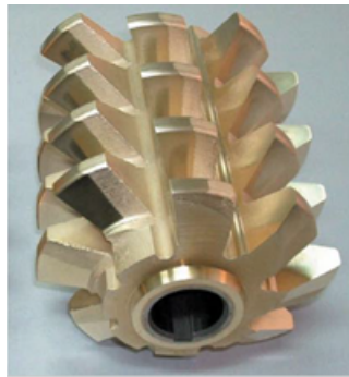
Figure 10. High-speed steel hob with multilayer 11x(TiN/ZrN) coating deposited by PVD arc plasma at Łukasiewicz-IAMT—with module m = 10 mm (Czechowski 2017)
