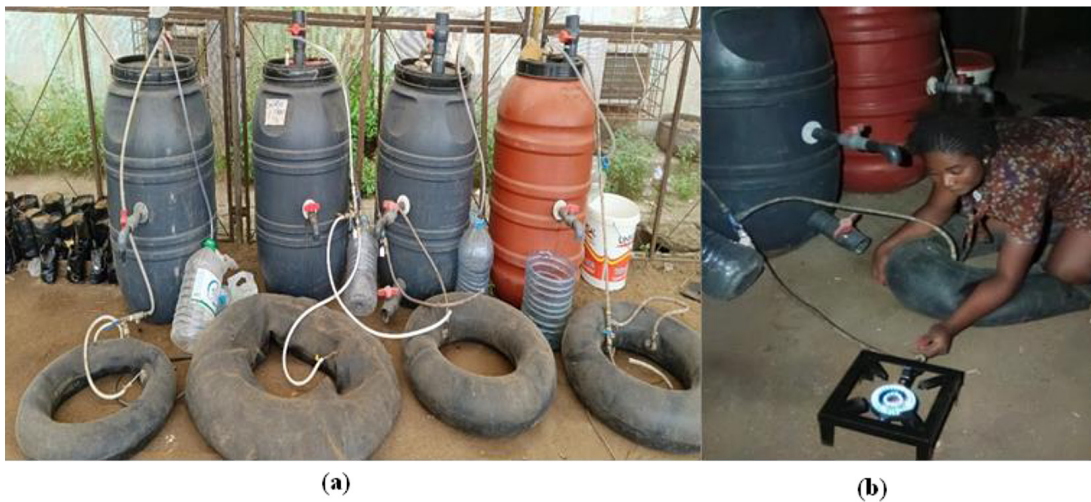
Figure 11. Final illustrations of the experimentation: a) air chambers filled with biogas; b) flames showing the combustion of biogas produced
