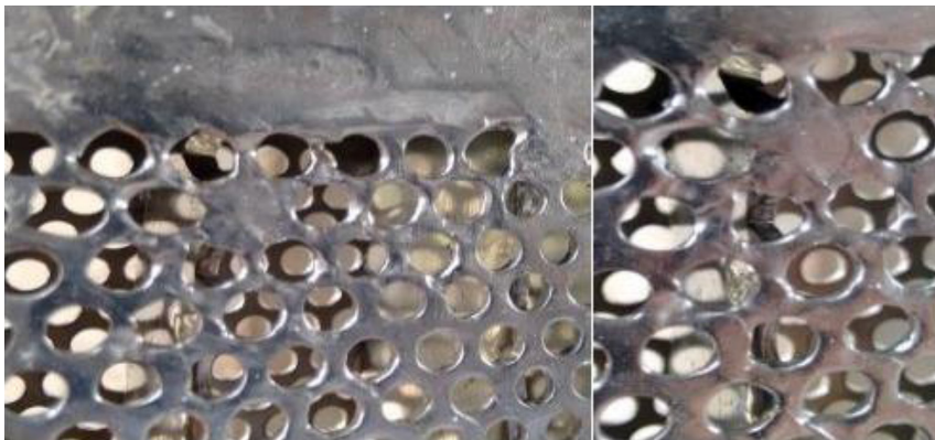
Fig. 4. Damage to the sector backing plate Source: Drytech Int.
