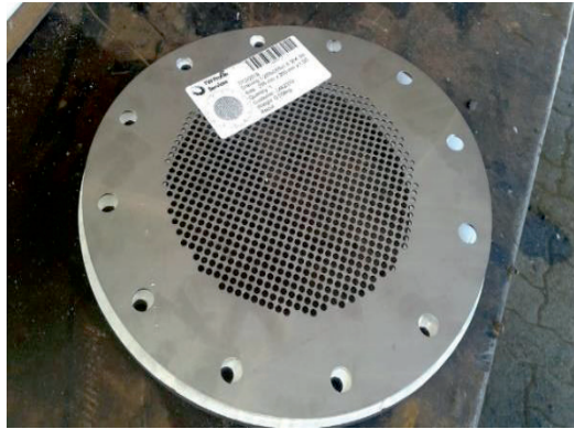
Fig. 9. Manufactured stainless-steel perforated backing plate Source: Drytech Int.
