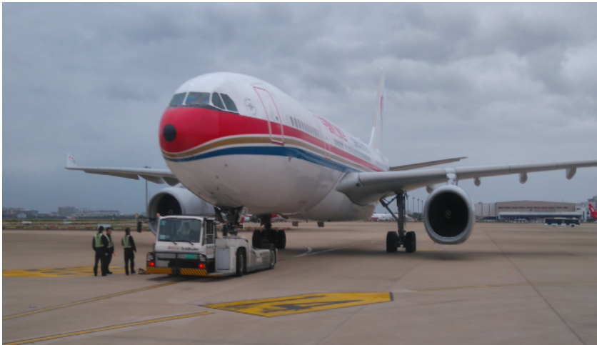
Fig. 1. A plane ready to be towed without a towbar; near the tug, people engaged in towing can be seen
