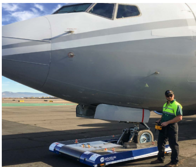
Fig. 2. Remotely-controlled electric tug; the operator with a control panel (visible in the figure) can move freely anywhere [4]
